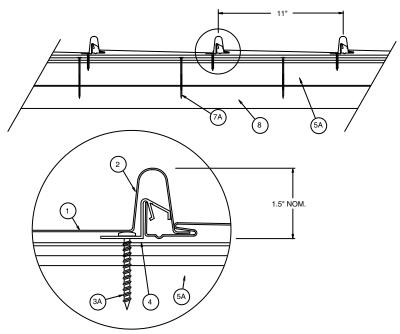
Metal Roof Deck Panels\* - No. 24 MSG min coated steel panels, 11 in. wide, \_ in. high at female side rib and 1-1/2 in. high at the male side rib. Panels continuous over three or more clips with no endlaps. A bead of sealant may be used at panel side joints.
